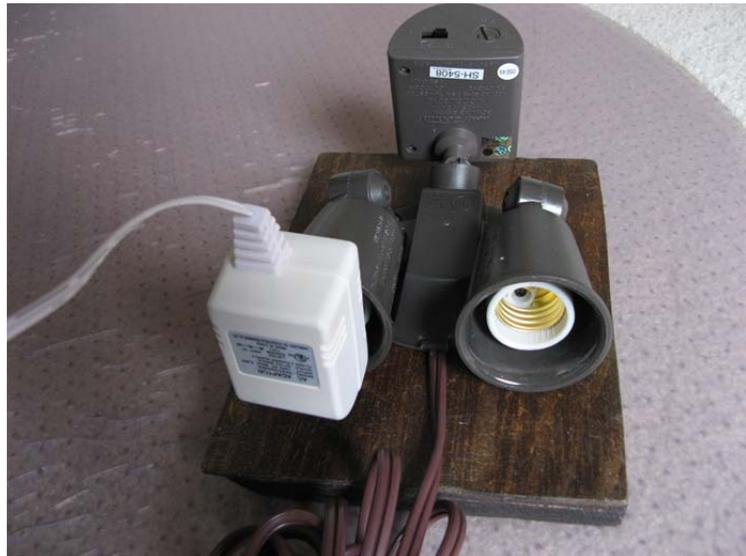
Now the sensor is ready. Move your hand in front of the sensor to test it. The prop should turn on for no more than 10 seconds, and then the sensor will reset itself. Experiment with the sensitivity dial to find the desired activation range.
