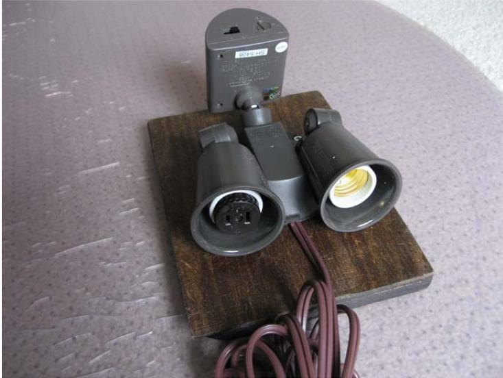
Face the two light sockets away from the sensor, tighten them into position, and attach the two electrical plug light socket adapters.
